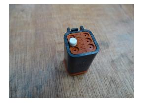
4.3. On the vehicle harness, throttle pedal connector (marked C021), on the top side of the connector you will see the cavities are named from left to right `A-F'.
