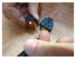
4.8. Repeat this process with the wires from cavities B, C, D, F, inserting each crimped terminal/wire into the Deutsch connector supplied, into cavities 2, 3, 4, 6 respectively.
