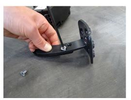
2.3. Fit mounting plate (107465) to the pedal assembly with socket c/sunk head screw (16473) 3 off.
